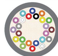
(representative cross-section with 24 fibers)
